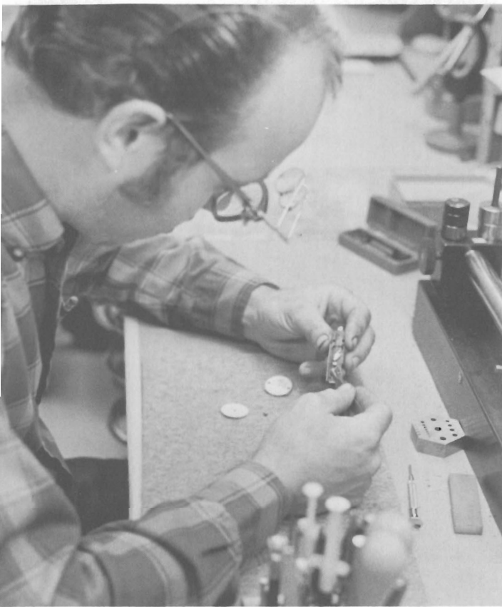
Evaluation and repair are important functions at the lab. "Fixed" gages that show wear have to be scrapped, but most adjustable gages can be restored. Here Rick Murray works on a dial indicator in need of adjustment.
