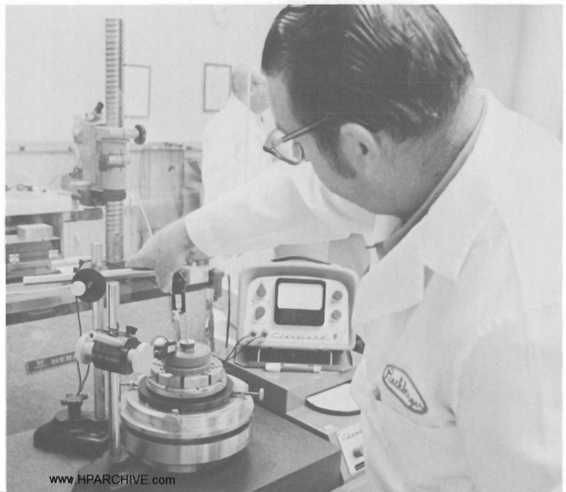
Ralph Richberger checks the roundness of a test arbor (precision shaft used in QA inspection) to within 10 millionths of an inch on special machine. Polar chart exaggerates and displays imperfections.
