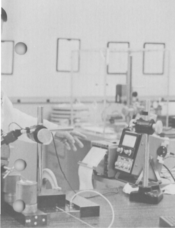
Lab manager Glenn Herreman (left) and Ed Duzowski check flatness of one surface of crystal to be used in HP laser interferometer. Most lab people have extensive experience as machinists, tool engineers, model makers or tool-and-die makers.
